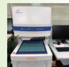
CNC image measuring instrument
