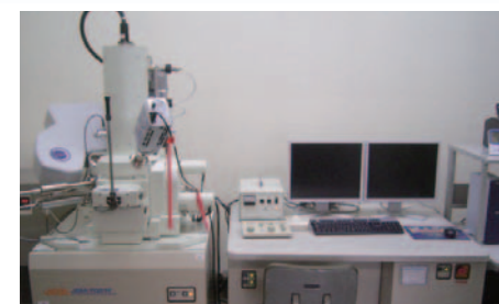
Field emission SEM with EDX and WDX systems
