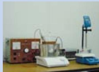
Hull Cell Testing Device
