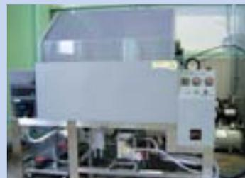
Salt Water Atomizing Testing Apparatus
